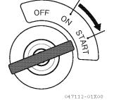
**4.** After the engine has started, release the starter switch key.
