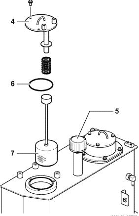
**12.** Put oil to the specified level through the oil supply port 5.
