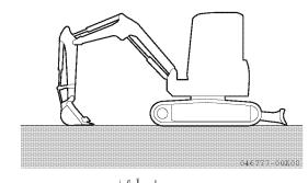
2. Lower the attachment onto the ground.
