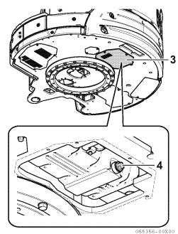
■ Checking the fuel level in the fuel tank and refueling
