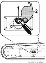
**6.** The tension can be adjusted until the clearance "a" is reduced to 0 in. (0 mm). If the tension is still loose after adjustment, the pin and the bush should be reversed or replaced because they are worn excessively. Ask your dealer to repair the track.
