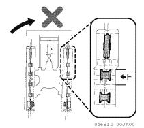
Traveling in reverse under this condition will cause the rubber track to come off.
