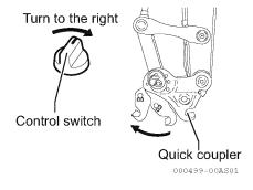
**7.** Only one of the bores allows the whole lock pin. Install the lock pin to that bore.
