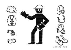
Take particular precautions when generating metal debris, when striking metal objects with a hammer or when cleaning components with compressed air.
