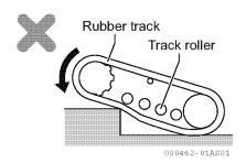
If the machine further travels in reverse, clearance may also be created between the track rollers and the idler and, the rubber track, causing the rubber track to easily come off.
