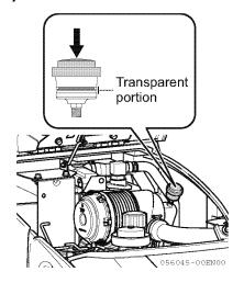
■ Checking and replenishing the engine oil
